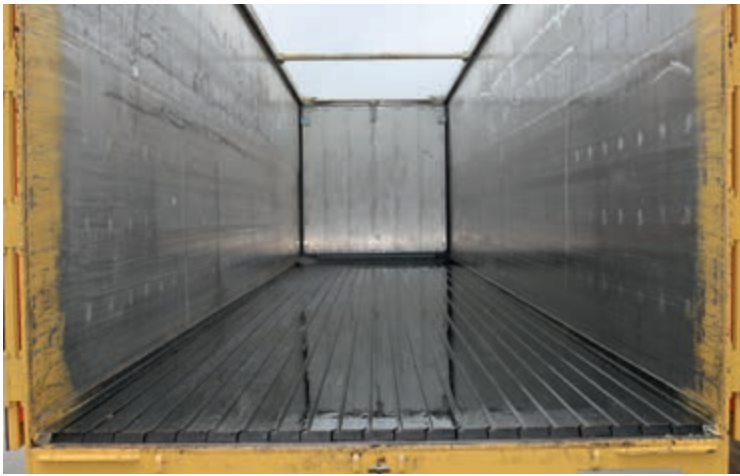
Sealless STEEL L-shape floor with an exceptional metallic coating for corrosion protection Magnelis®.
