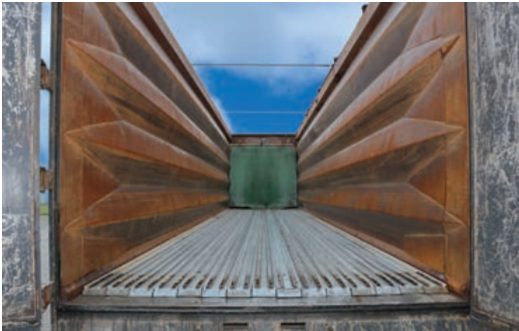
XHDI aluminum Impact floor with high tensile steel inlay wear protection.
