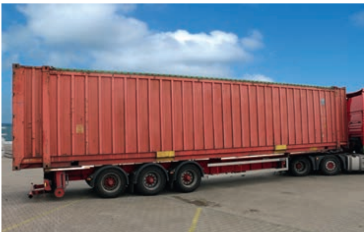
45ft high cube sea container with perimeter mount Cargo Floor.
