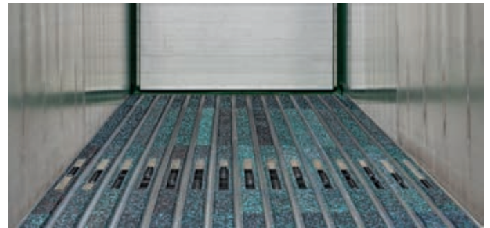
Only cut outs in subdeck for connecting drive-shoes to slat.
