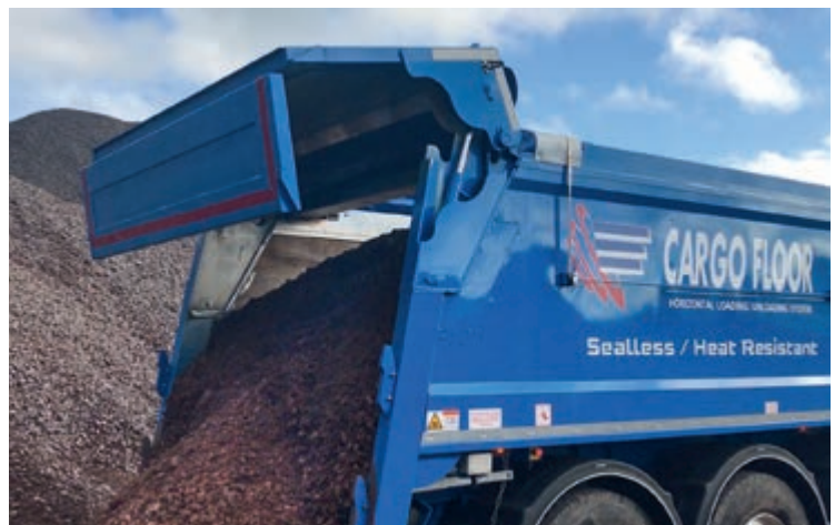
Sealless aluminum heavy duty floor for aggregates 'roadworks'.
