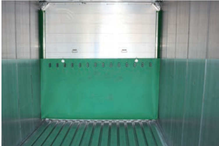
Moving headboard for easy and clean unloading!
